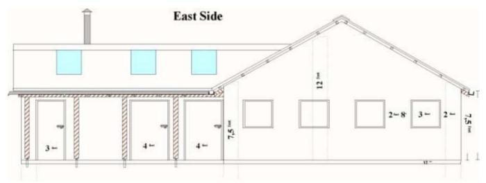
**Doors** shall be wider than in normal houses to give easy access for wheel chair, stretcher and moving in and out furniture. The Door Frames shall have **no bottom frame** to make easy access for wheel chair and to make cleaning more easily. Therefore anchors shall be prepared for the walls and iron bars to be fixed in the RCC before pouring concrete.
