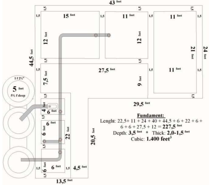
Before the cement work on RCC and floor is initiated, it is very important that the construction site is very **well prepared**. Both fundament and floor shall be prepared at the same time, so all the concrete work can be done within few days so fundament and floor will be constructed in one piece.
