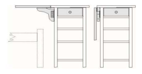
over the bed and the legs of the sick person for better access to eat and others. A strong wooden plate under the folding table top shall for that purpose with hinges be turned out to support the table top. Don't start this woodwork before the beds are completed, so the right height and functionality can be measured and the result can be tested on the spot.
