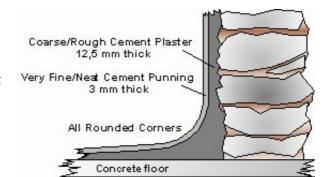
that will make i easy to keep clean. First a 12,5 millimeter thick layer of **1 cement**: **4 sand** shall be plastered all over the floor and all the walls from bottom to top. And remember that all corners shall be strongly rounded. Finally these surfaces shall be **punned** with a thin layer (3 mm) of **2 cement**: **1 very fine sand**. The sand has to be extremely fine; otherwise it is better to use only cement for punning.
